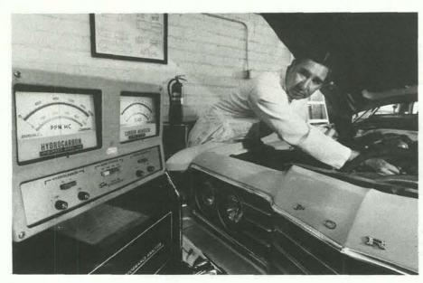
TUNE 'EM UP—That's the word from and job of Ernie Marquez (8718) who recently performed that chore on the 100 vehicles assigned to Area III. He adjusted carburetors and timing and replaced air filters and points to ensure lowest possible gasoline consumption and harmful emissions.
